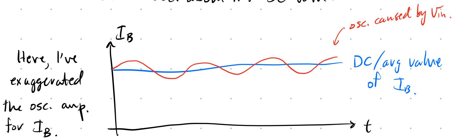
Recall that small changes in  $I_B$  result in large changes to  $I_c$  (current amplifier)
