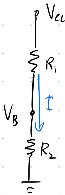
$$V_{cc} - I(R_1 + R_2) = 0$$
