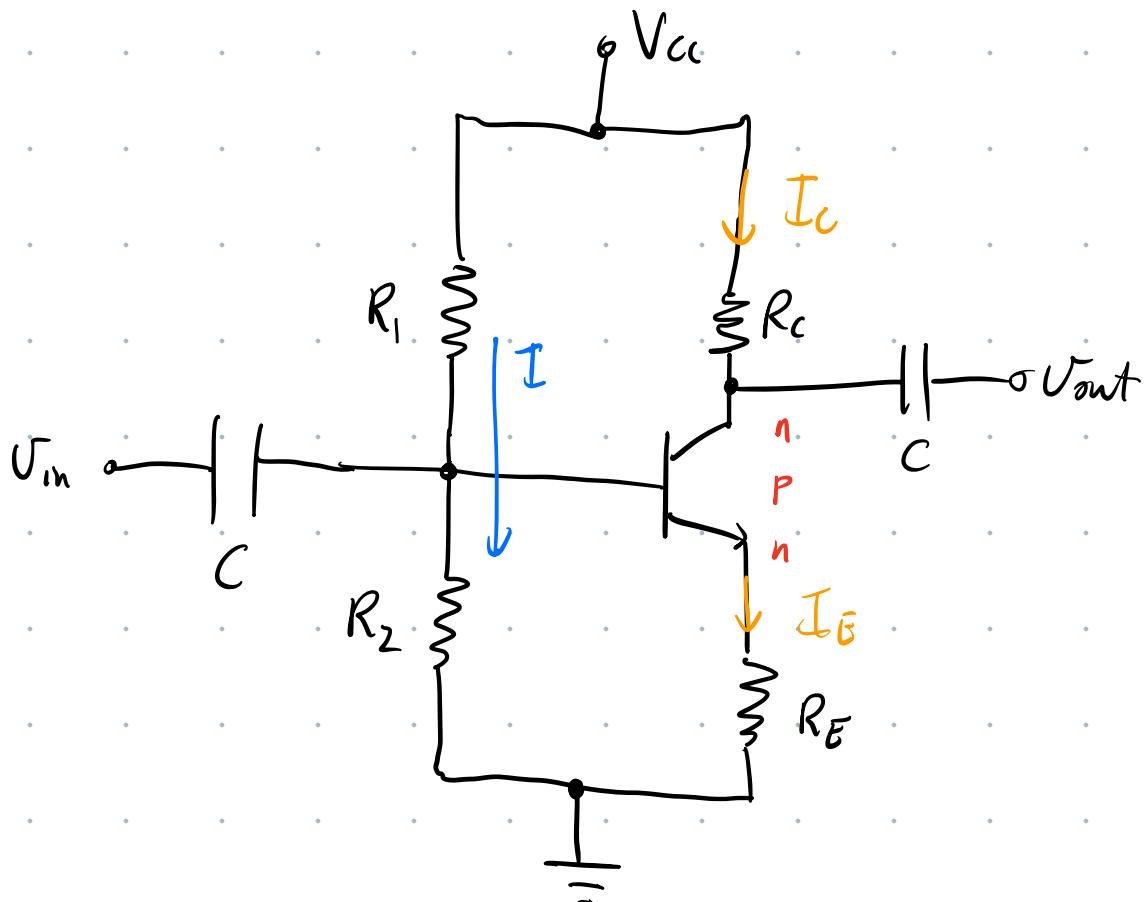
$V_{cc}$ ,  $R_1$ , &  $R_2$  are chosen to bias the transistor
